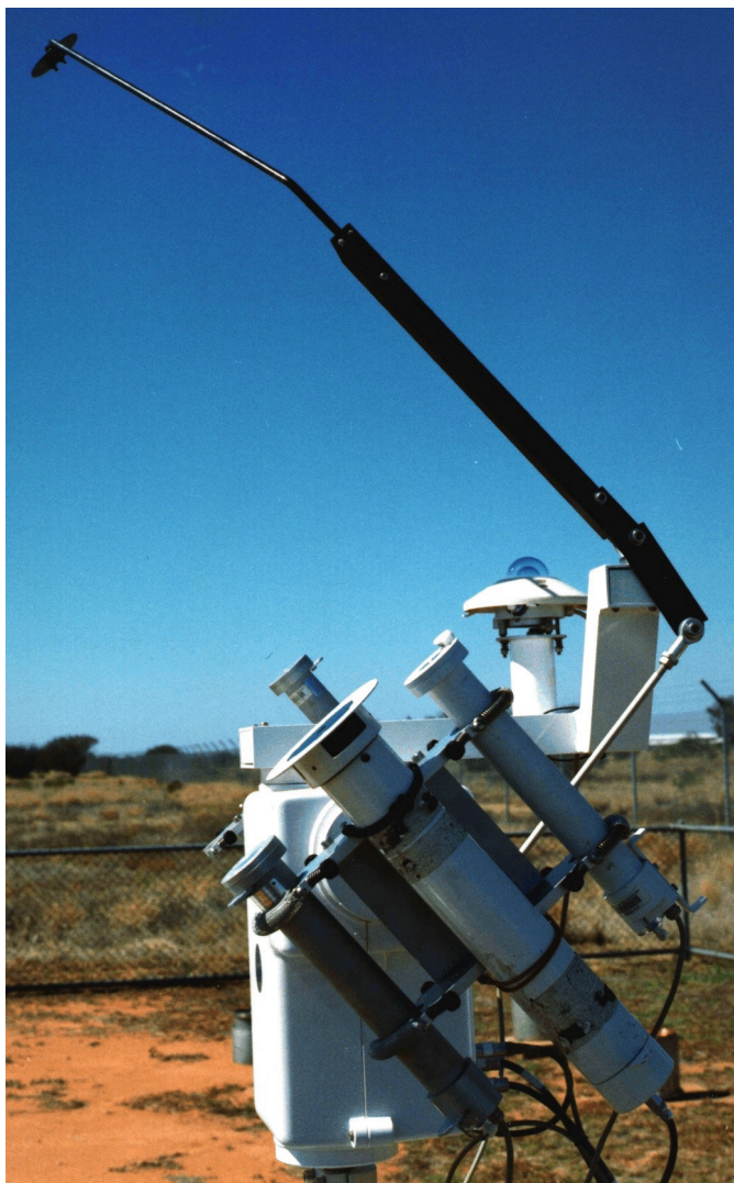
Figure 4.5. Australian active tracker used for both diffuse and direct beam measurements. This tracker is shading a single pyranometer, and pointing two normal incidence pyrheliometers and a GAW PFR sunphotometer on one side of the tracker and another pyrheliometer on the far side of the tracker. An active-eye is also situated on the far side of the tracker. (Courtesy Bureau of Meteorology, Australia)
